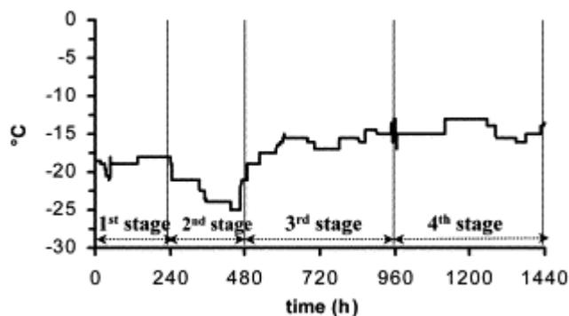
Fig. 3. Indicative temperature profile of distribution of frozen vegetables in the real chill chain (total distribution time 60 days) (Giannakourou and Taoukis, 2003).
