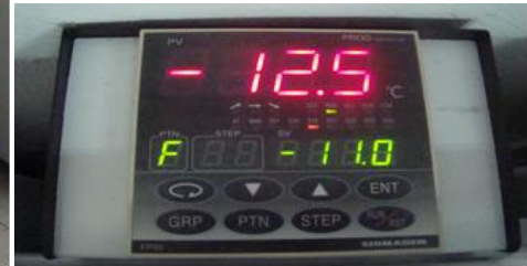
Figure 12. WHIRLPOOL AFG543 freeze cabinet (left) and display detail (right)
