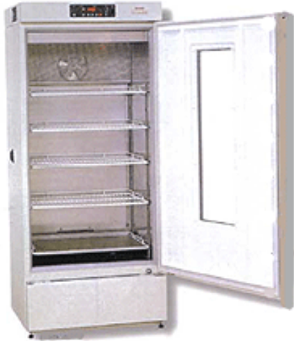
Figure 10. SANYO MIR-253 cooled incubator
