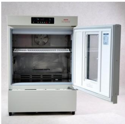
Figure 8. SANYO MIR-153 cooled incubator
