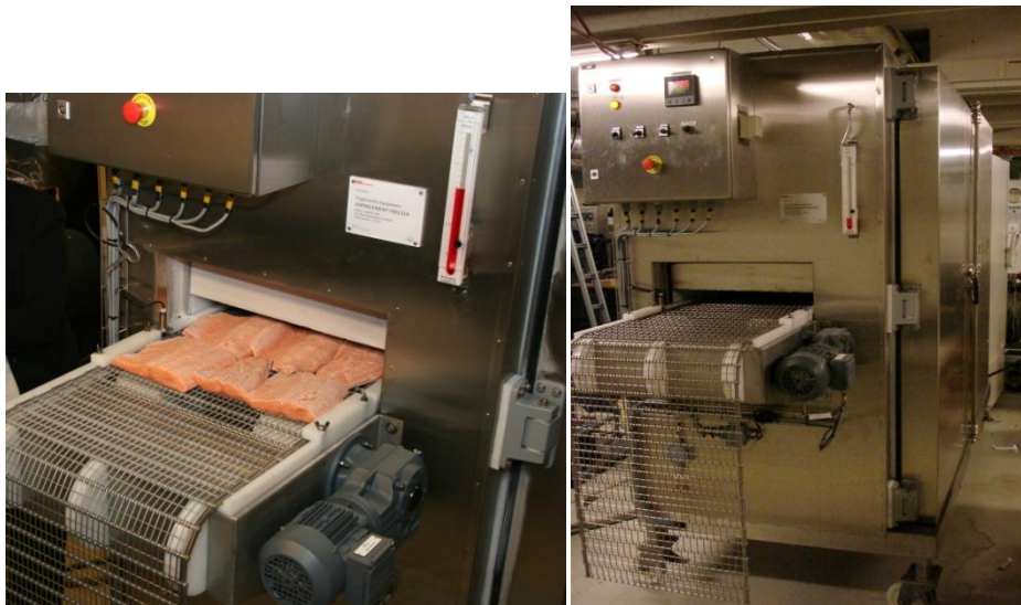
Figure 6. Impingement freezer at SINTEF
