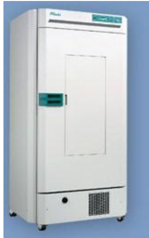
Figure 3. Chilling cabinet at SINTEF
