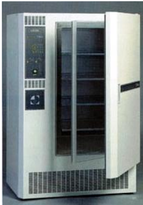
Figure 1. The temperature controlled incubator (Termaks, series 6000)
