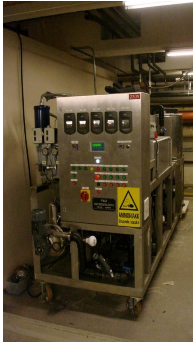
Figure 7. Mobile ice slurry unit using sea water and having a 1000 L buffer tank
