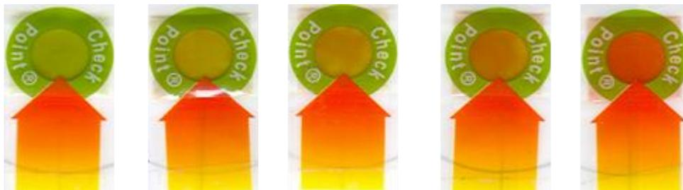
**Picture 7.** Response scale of enzymatic CheckPoint® TTI from green at time of application (left) to orange-red (right) indicating the end of shelf life.
