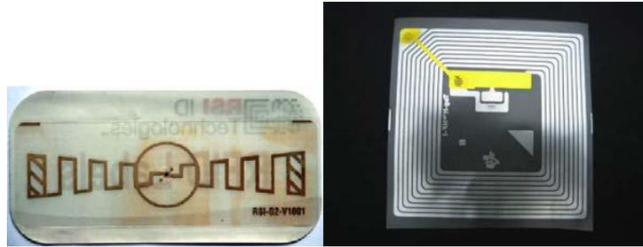
**Picture 6.** Examples of RFID tag: Left: Courtesy of Behnam Jamali, the University of Adelaide; right: Courtesy of Mark Lohmann, CHILL-ON project (Estrada-Flores and Tanner, 2008)
